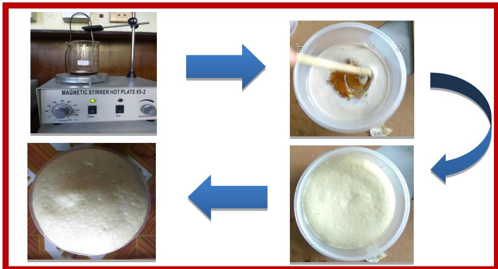
**Figure 3:** Schematic of polyurethane-TiO<sub>2</sub> composites foam production
